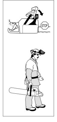
4 To release the chain brake pull the front hand guard backwards, towards the front handle.
